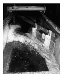
FIGURE 1: Photograph of the test section looking downstream from above;  $\theta = 13.4^{\circ}$ ,  $\phi \approx 15^{\circ}$ , U = 2.45m/s, d = 11.45cm, and  $\mathbf{F} = 2.31$ .
