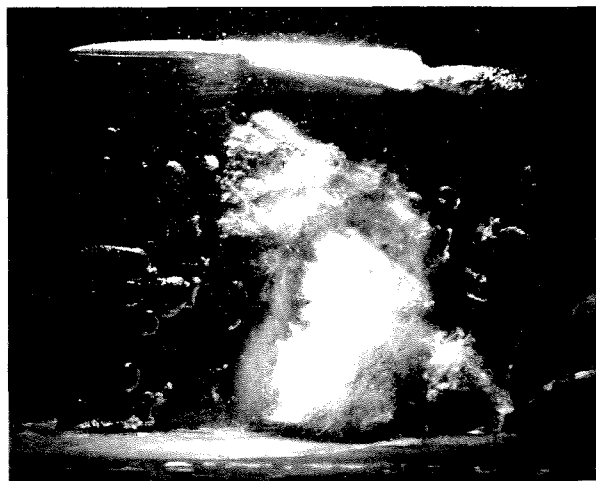
Figure 2: Between cavitation cycles: the cloud at the right is collapsing and beginning to disperse, while travelling bubble cavitation can already be seen near the leading edge just prior to forming a new sheet cavity. \sigma = 1.0 , k = 0.8 , TAC = 4 - 5ppm , \alpha = 7.9^\circ ( \alpha increasing).
