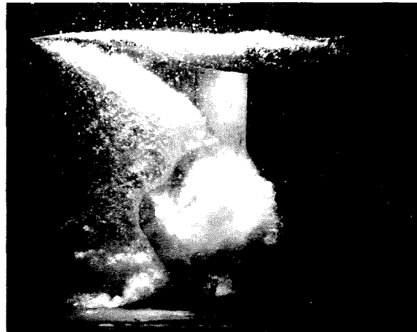
Figure 1: Cloud cavitation on an oscillating hydrofoil. The photograph on the left is without air injection, \sigma = 1.2 , k = 0.9 , \alpha = 10.3^\circ ( \alpha decreasing). The photograph on the right has a normalized air flow rate of q = 2.2 \times 10^{-4} , with \sigma = 1.2 , k = 0.8 , \alpha = 7.4^\circ ( \alpha decreasing).
