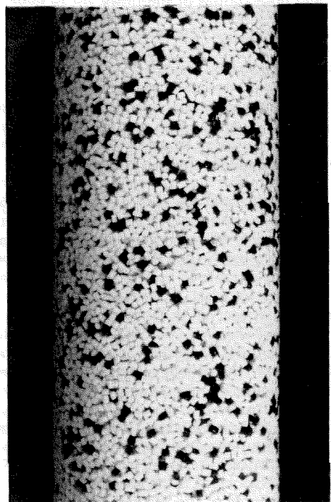
Fig. 12 Solids-water plug flow of 55 percent volume fraction
