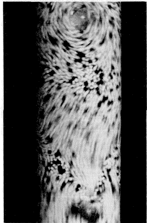
Fig. 16 Three component flow of 30 percent solids volume fraction and 15 percent air volume fraction, showing large vortex structure. 1/30 second exposure was used.
