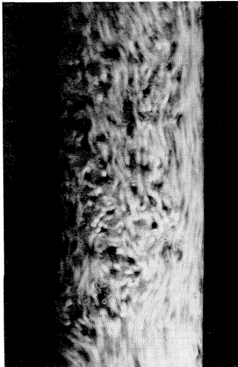
Fig. 15 Three component flow of 12 percent solids volume fraction and 15 percent air volume fraction, showing the small scale structure of disperse flow. 1/30 second exposure was used.
