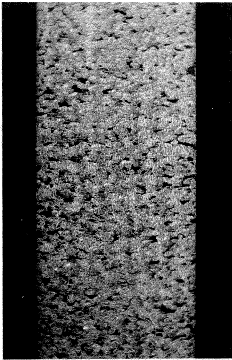
Fig. 6 Bubbly-air water flow of 8 percent volume fraction
