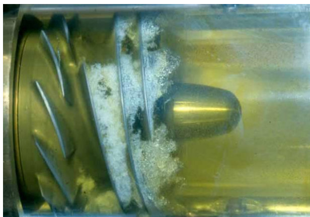
Cavitating model of the Low Pressure Liquid Oxygen Pump in the Space Shuttle Main Engine [13]
