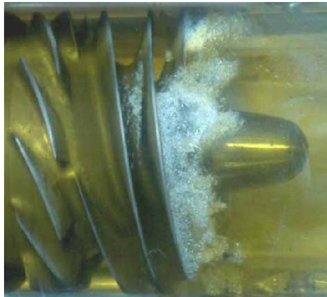
Figure 1. Scale model of the low pressure liquid oxygen pump impeller for the Space Shuttle Main Engine (SSME) in moderate cavitating conditions in water.
