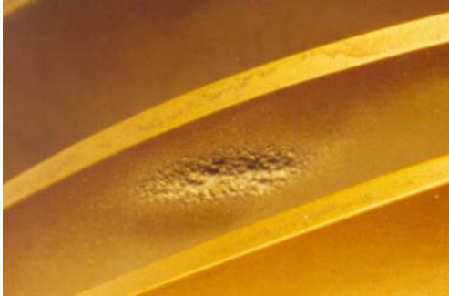
Figure 10. Photograph of localized cavitation damage on the blade of a mixed flow pump impeller made from an aluminum-based alloy.
