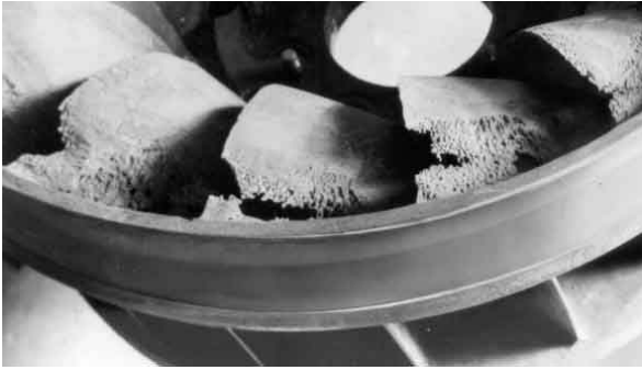
Figure 9. Major cavitation damage to the blades at the discharge from a Francis turbine.
