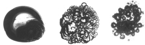
Figure 8. Photographs of an ether bubble in glycerine before (left) and after (center and right) a collapse and rebound, both bubbles being about 5-6mm across [29].
