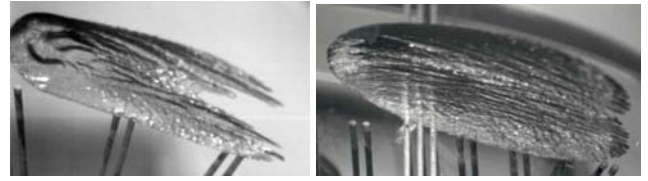
Figure 14. Typical cavitation events from the scaling experiments of Kuhn de Chizelle et al. [41] showing transient bubble-induced patches, the left one occurring on a 50.8cm diameter Schiebe headform at \sigma = 0.605 and a speed of 15m/s, the right one on a 25.4cm headform at \sigma = 0.53 and a speed of 15 m/s. The flow is from right to left. The lifesize widths of the photographs are 6.3cm (left) and 7.6cm (right).
