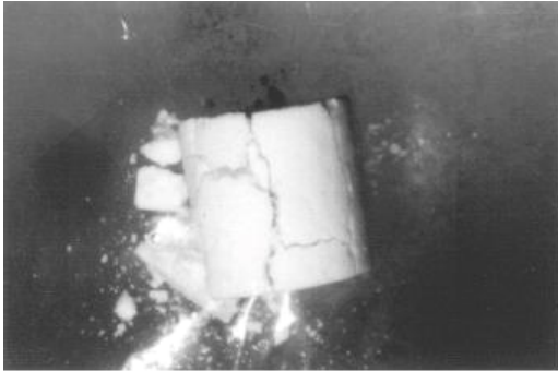
Figure 6. Artificial stone fractured by shockwave lithotripsy [23].
