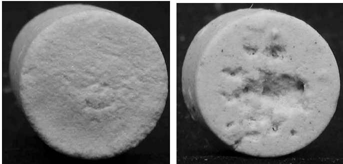
Figure 7. New and damaged artificial renal stone (courtesy of Erin Hatt, Dept. of Anatomy and Cell Biology, Indiana University).
