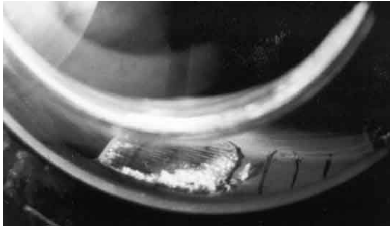
Figure 5.9. Blade cavitation on the suction surface of a blade in a centrifugal pump. The relative flow is from left to right and the cavity begins at the leading edge of the blade which is toward the left of the photograph. From Sloteman, Cooper, and Graf (1991), courtesy of Ingersoll-Dresser Pump Company.
