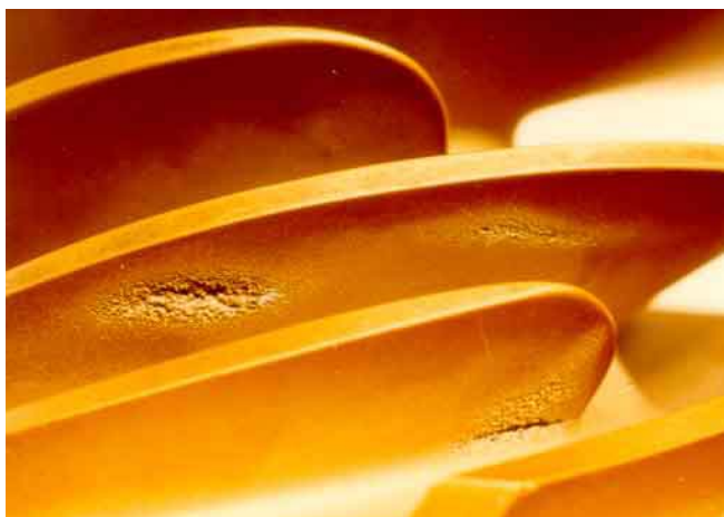
Figure 6.3. Photograph of localized cavitation damage on the blade of a mixed flow pump impeller made from an aluminium-based alloy.
