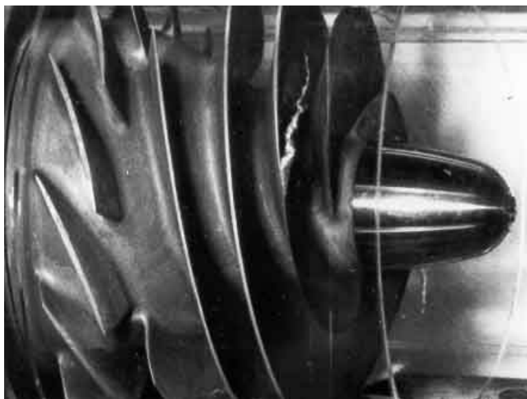
Figure 5.7. Tip vortex cavitation on Impeller IV, the scale model of the SSME low pressure LOX turbopump (see figure 2.12) at an inlet flow coefficient, \phi_1 , of 0.07 and a cavitation number, \sigma , of 0.42 (from Braisted 1979).
