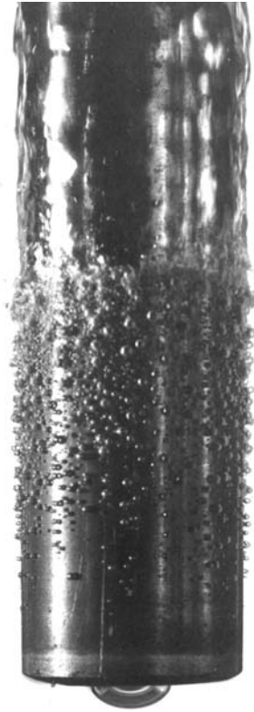
Figure 6.14: The evolution of convective boiling around a heated rod, reproduced from Sherman and Sabersky (1981).
