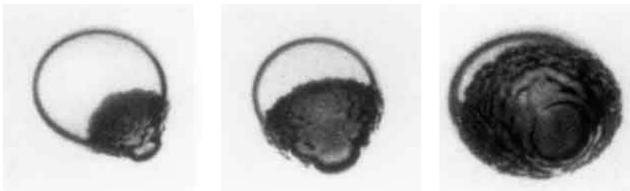
Figure 6.8: Typical photographs of a rapidly growing bubble in a droplet of superheated ether suspended in glycerine. The bubble is the dark, rough mass; the droplet is clear and transparent. The photographs, that are of different events, were taken 31, 44, and 58 \mu s after nucleation and the droplets are approximately 2 mm in diameter. Reproduced from Frost and Sturtevant (1986).
