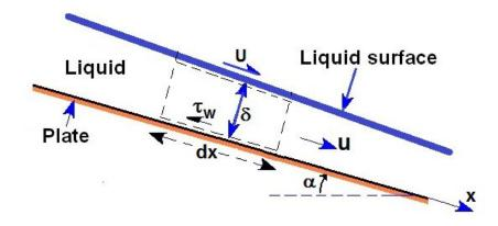
Assuming a velocity profile and wall shear stress similar to that for a turbulent boundary layer on a flat plate:
