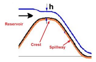
Since the flow downstream of the crest of the spillway is supercritical it follows that the flow at the top of the crest must be critical and therefore the velocity of flow at the crest is  $u_c = (gh)^{1/2}$  where h is the depth of the water at the crest. Therefore the flow rate Q is  $Q = bh(gh)^{1/2}$  where b = 15m is the breadth of the crest. It follows that  $Q = 7.72m^3/s$ .
