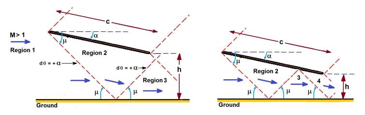
(a) If c is equal to  $2h/\tan\mu$  then the Mach wave reflected by the wall will precisely impinge on the trailing edge if
