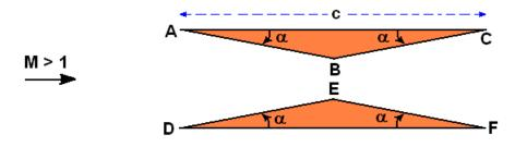
Since the angles BDF and EAC are both equal to the Mach angle,  $\mu = \arcsin(1/M)$ , Mach waves emanating from the points A and D will impinge directly on the vertices E and B respectively and since the flows in the regions 2 are compressed by the angle  $\alpha$  it follows that the pressures in the regions 2 will be
