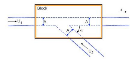
Consider a control volume consisting of the block. Since the fluid is incompressible the velocity of the flow out through the right hand opening is  $U_1 + U_2$ . Therefore the net momentum flux out of the control volume (assuming uniform velocity profiles) is
