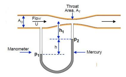
pressure taps are located upstream of the nozzle and at the throat; these are connected to a water/mercury manometer as shown. When the water is flowing through the device, the manometer levels differ by an elevation, h.
