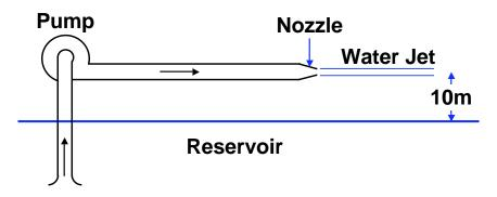
A modified Bernoulli equation applied between a point on the external free surface outside the submerged pipe (point 1) and the jet after it emerges from the nozzle (point 2) yields
