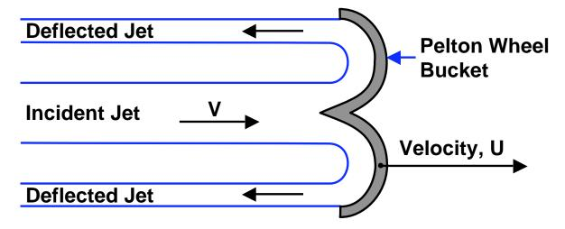
viscous effects, Bernoulli's equation along the streamline connecting the incident jet to one of the deflected jets yields:
