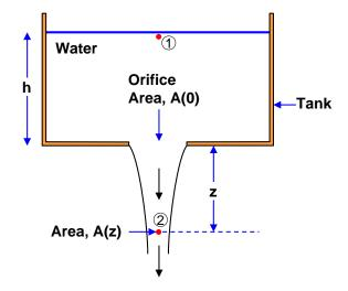
the water in the tank as point 1 and a point a distance z below the orifice in the bottom of the tank as point 2, the steady form of Bernoulli's equation yields:
