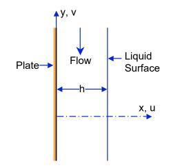
Consider a control volume spanning the whole layer, with unit height in the y direction and unit depth normal to the diagram. The weight of the liquid in this control volume is  $\rho gh$  and this must be balanced by the upward shear force at the wall (since the flow is steady and since the pressures acting on the top and bottom of this control volume are the same). Since the velocity in the y direction is
