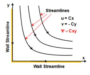
$$\omega = \frac{\partial v}{\partial x} - \frac{\partial u}{\partial y} = 0 \tag{1}$$
