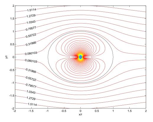
d) For  $r \gg r_0$  it follows that  $u_r \to U \cos \theta$  and  $u_{\theta} \to -U \sin \theta$  and consequently the magnitude of the flow velocity is  $|\vec{u}| = \sqrt{u_r^2 + u_{\theta}^2} = U$  and the direction is in the  $\theta = 0$  direction. Consequently the flow far away is a uniform stream of magnitude U in the  $\theta = 0$  direction.
