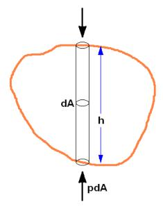
acting on a body immersed in a fluid as shown above. Consider a vertical cylindrical element of crosssection, dA, and length, h, and denote the pressure in the fluid at the lower end by p. Then the pressure at the top end will be
