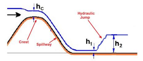
If the depth of the flow at the bottom of the spillway,  $h_1 = 0.1m$ , find the depth of the flow downstream of the hydraulic jump,  $h_2$ . Neglect frictional effects upstream of the jump.
