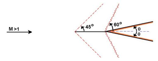
Then, a second experiment is carried out after a very slender probe has been attached to the front of the wedge as shown in the sketch. A Mach wave is observed to occur, inclined at  $45^{\circ}$  to the oncoming stream. What is the wedge angle,  $\delta = 2\theta$ ?
