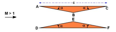
The oncoming stream is parallel with the sides AC and DF. The flow is to be analyzed using the supersonic theory for small angles of turn. If the angles BDF and EAC are both equal to the Mach angle,  $\mu = \arcsin(1/M)$ , find the drag coefficient for the foils.
