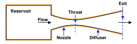
Assume the gas behaves like air  $(R = 280 \ m^2/s^2 \ K^{\circ}, \gamma = 1.4)$ . The flow reaches critical conditions at the throat, is subsonic upstream of the throat and supersonic in the divergent section between the throat and the exit. The pressure at exit is atmospheric  $(10^5 \ kg/m \ s^2)$  and the supersonic flow at the exit is travelling at M = 2.5. Find:
