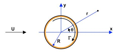
Here the circulation,  $\Gamma$ , is defined as positive in the clockwise direction. That is to say we have used the normal airfoil sign convention. This simulates the flow due to clockwise rotation of the cylinder.
