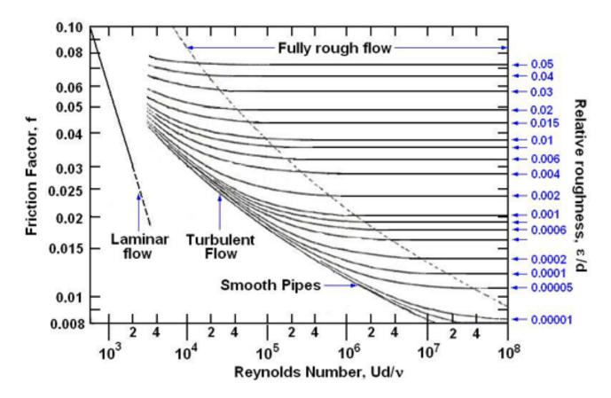
[Note that the friction factor,  $f = d(-dp/dx)/\frac{1}{2}\rho U^2$ ,  $Re = dU/\nu$  where d is the diameter and U is the volumetric average velocity of flow.]
