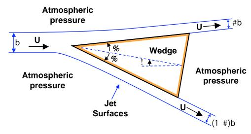
The angle of attack,  $\alpha$ , of the wedge is also defined in the sketch. The result is that the single incident jet is divided into two jets both of which leave the back edges of the wedge with the velocity, U. The widths of the two departing jets are  $\beta b$  and  $(1 - \beta)b$  as indicated in the figure. It is assumed that the flow is planar and that the pressure in surrounding air is everywhere atmospheric.
