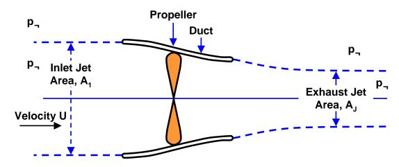
The characteristic of the propeller is such that it produces a total head rise,  $\Delta H$ , which is related to the volume flow rate, Q, by
