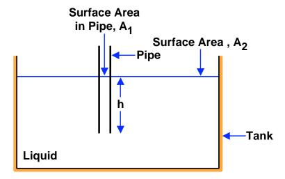
Neglecting all viscous effects and all inertial effects except for that of the water inside the pipe (the inertial effects in the water outside the pipe will be small since  $A_2^{>>}A_1$ ) find the natural period of oscillation of the water rising and falling in the pipe. The water is assumed incompressible. The answer should involve  $A_1$ ,  $A_2$ , h and g.
