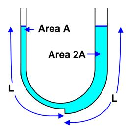
Find the natural frequency of manometer oscillations in this U-tube, denoting the acceleration due to gravity by g.
