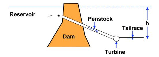
The frictional losses in the penstock (the pipe leading to the turbine) and the tailrace are represented by the loss coefficient, k, based on the mean velocity, U, in those pipes (which have the same cross-sectional area, A). The flow discharges to atmospheric pressure at the exit from the tailrace. The water density is denoted by  $\rho$  and the acceleration due to gravity by g.
