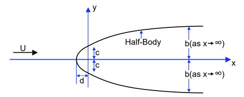
If the strength of the source is denoted by q find the dimensions b, c and d as shown in the sketch.
