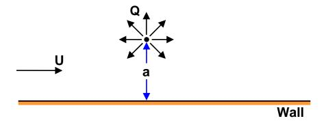
The fluid injection can be represented by a planar or line source and the flow remains planar. Determine the particular volume flow rate, Q, above which the injected fluid reaches the wall. The answer involves U and a.
