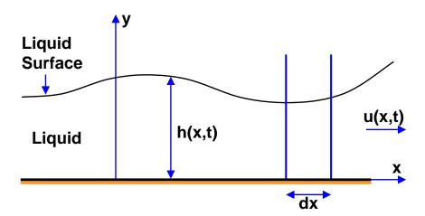
The depth, h(x,t), is a function of x and time, t. Examine an Eulerian element of width, dx, as shown above (it extends from y = 0 to  $y = \infty$ ) and assume that the velocity, u(x,t), of the water in the positive x direction is **independent of** y. Then utilize conservation of mass to obtain a partial differential equation connecting the depth, h(x,t), and the velocity, u(x,t). Neglect surface tension. [This is one of the equations of what is known as "shallow water wave theory".]
