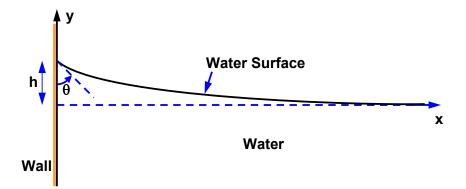
The surface tension of the liquid surface is denoted by S and the contact angle with the wall by  $\theta$ . Find the equation of the water surface in the form y = f(x); the function should contain the quantities S,  $\theta$ ,  $\rho$  and the acceleration due to gravity, g. To simplify the problem assume that the curvature of the water surface can be approximated by  $d^2y/dx^2$ . Find the height, h, in terms of S,  $\theta$ ,  $\rho$  and g.
