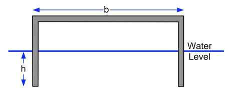
As indicted in the figure, the vertical sides are submerged to a depth h and the width of the channel section is b. If the center of mass of the channel section happens to lie on the waterline find the particular value of the ratio b/h above which this floating configuration is stable.
