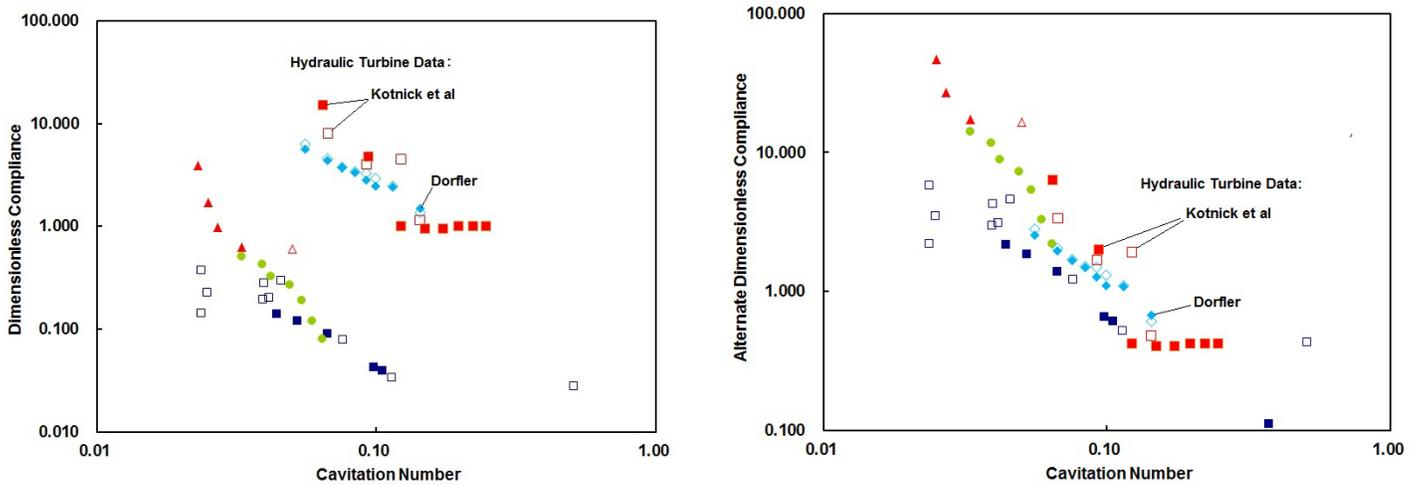
Figure 2: The dimensionless compliance,  $C'$  (left), and the dimensionless compliance,  $C''$  (right) plotted versus the cavitation number,  $\sigma$ , for many inducer pumps (see Section Nr<sub>q</sub>) and for the data from Dorfler (2018) and Manderla *et al.* (2016) for Francis turbines.
