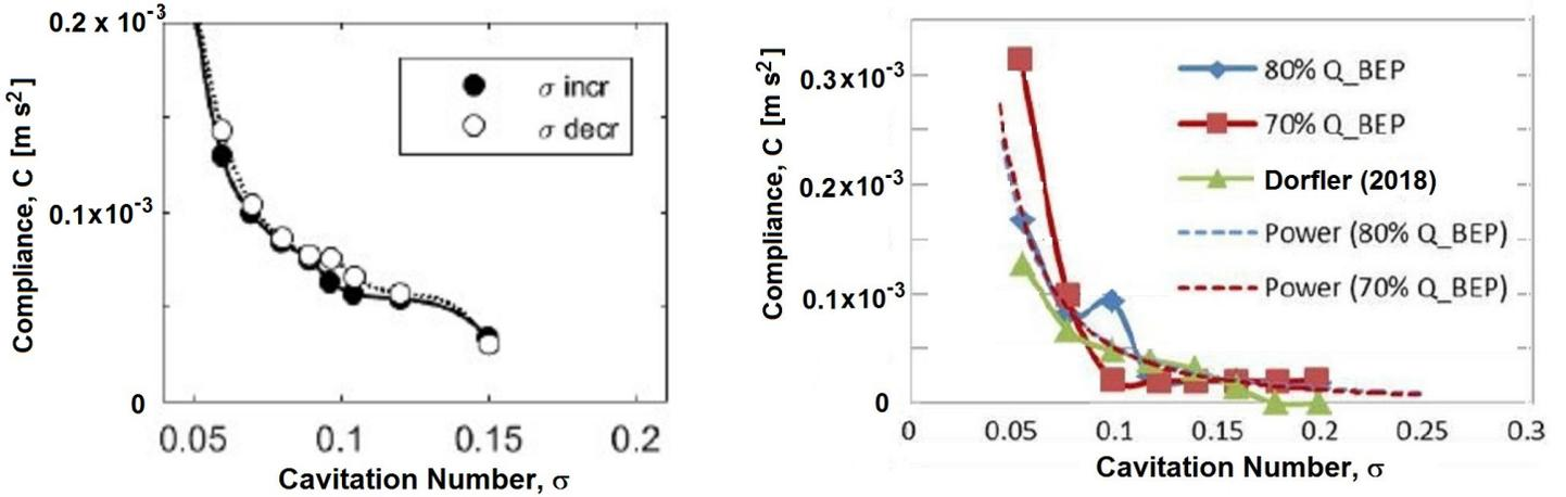
Figure 1: Compliances for a cavitating Francis turbine as a function of cavitation number, derived from experimental observations by Dorfler (2018) (left) and by Manderla *et al.* (2016) (right).
