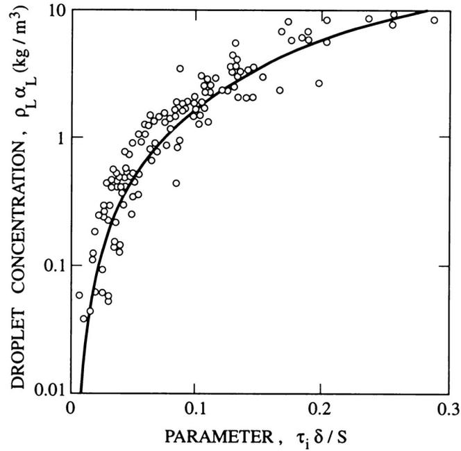
Figure 3: The mass concentration of liquid droplets in the gas core of an annular flow,  $\rho_L \alpha_L$ , plotted against  $\tau_i \delta / S$ . From Hutchinson and Whalley (1973).
