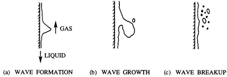
Figure 2: Sketch illustrating the ejection of droplets by wind shear in annular flow in a vertical pipe. From Hutchinson and Whalley (1973).
