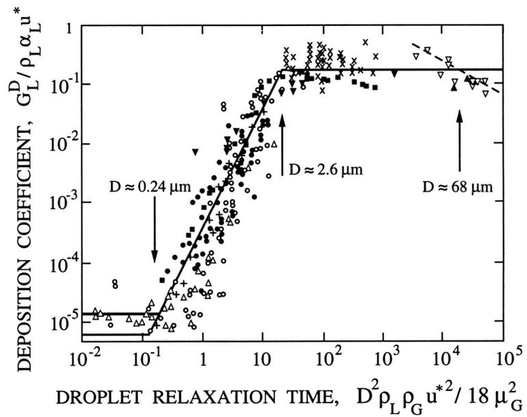
Figure 4: The dimensionless deposition mass transfer coefficient,  $G_L^D / \rho_L \alpha_L u^*$ , for vertical annular flow plotted against a dimensionless relaxation time for the droplets in the core,  $D^2 \rho_L \rho_G u^{*2} / 18 \mu_G^2$ . A summary of experimental data compiled by McCoy and Hanratty (1977).
