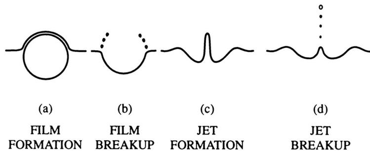
Figure 1: Stages of a bubble breaking through a free surface.
