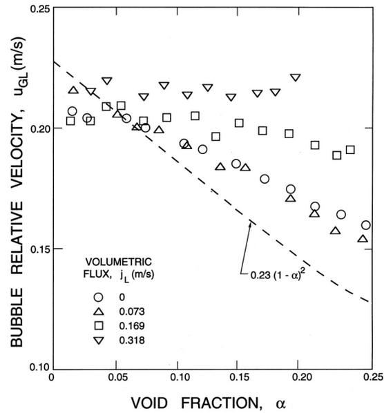
Figure 3: Data indicating the variation in the bubble relative velocity,  $u_{GL}$ , with the void fraction,  $\alpha$ , and the overall flow rate (as represented by  $j_L$ ) in a vertical, 10.2cm diameter tube. The dashed line is the correlation of Wallis, equation (Nel8). Adapted from Bernier (1982).
