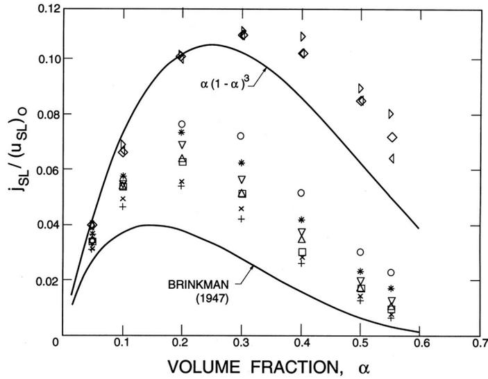
Figure 2: The drift flux,  $j_{SL}$  (normalized by the velocity  $(u_{SL})_0$ ) corresponding to the relative velocities of figure 1 (see that caption for codes).
