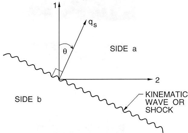
Figure 1: A two-dimensional kinematic wave or shock.
