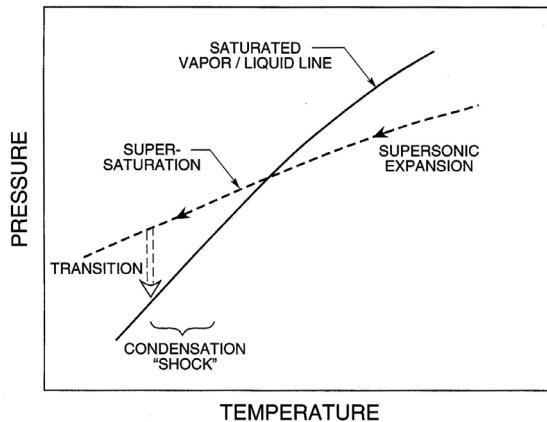
Figure 1: The occurrence of condensation during expansion in a diffuser.
