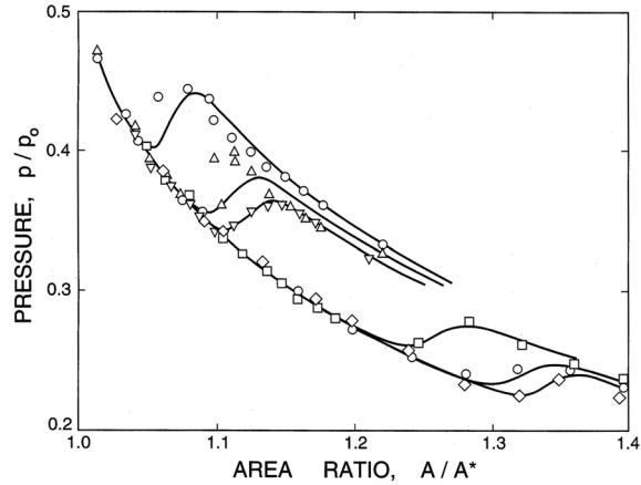
Figure 2: Experimental pressure profiles through condensation *fronts* in a diffuser for six different initial conditions. Also shown are the corresponding theoretical results. From Binnie and Green (1942) and Hill (1966).
