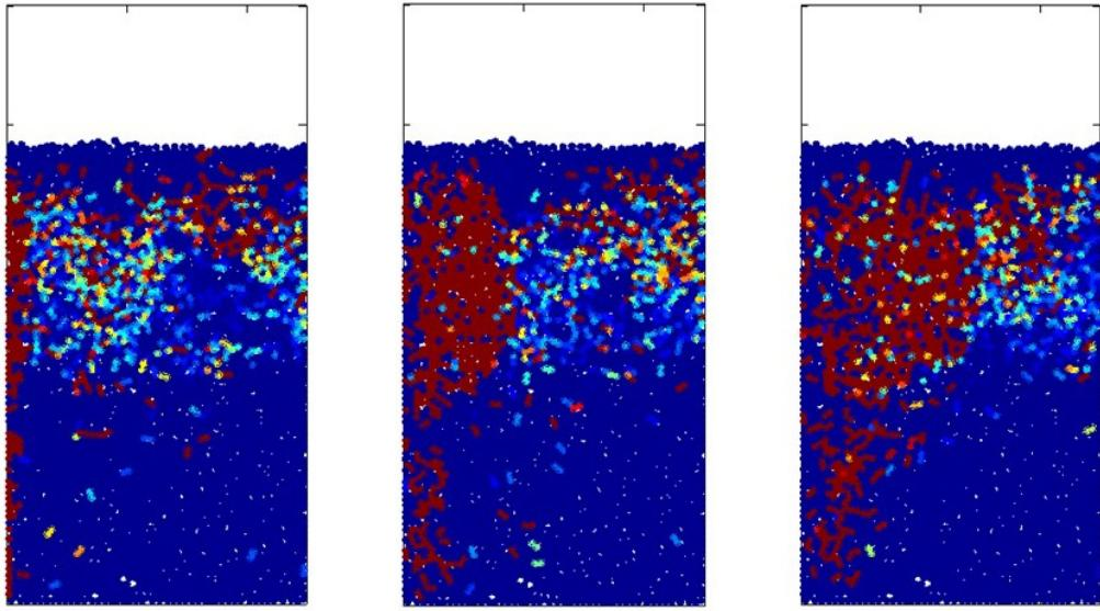
Figure 10: Transmission of a pressure wave in a shaken granular bed for three consecutive moments in time. The three images were captured at a moment in the shaking period when the upper particle layers are compressed while the lower particle layers are loose. From Hostler (2004).
