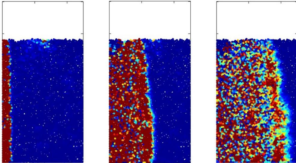
Figure 9: Transmission of a pressure wave in a static granular bed for three consecutive moments in time. From Hostler (2004).
