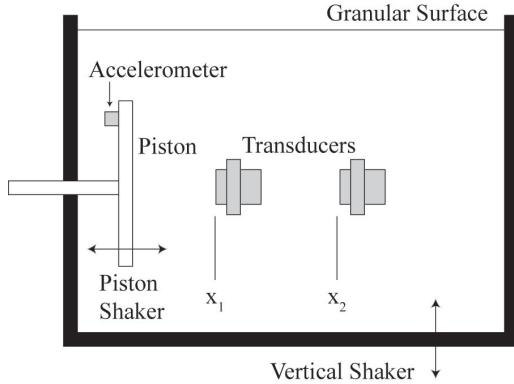
Figure 1: Schematic of wave propagation experiments. From Hostler and Brennen (2005).
