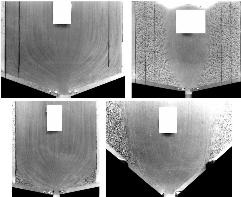
Figure 2: Long exposure photographs of typical granular flows in hoppers showing the streamlines in the flowing material. Top left: flow of sand without stagnant regions ( $H/W = 3.3$ ). Top right: a funnel flow of rice. Bottom left: flow of sand with stagnant corners ( $H/W = 1.6$ ). Bottom right: funnel flow of sand ( $H/W = 1.16$ ). From Nguyen *et al.*(1980).
