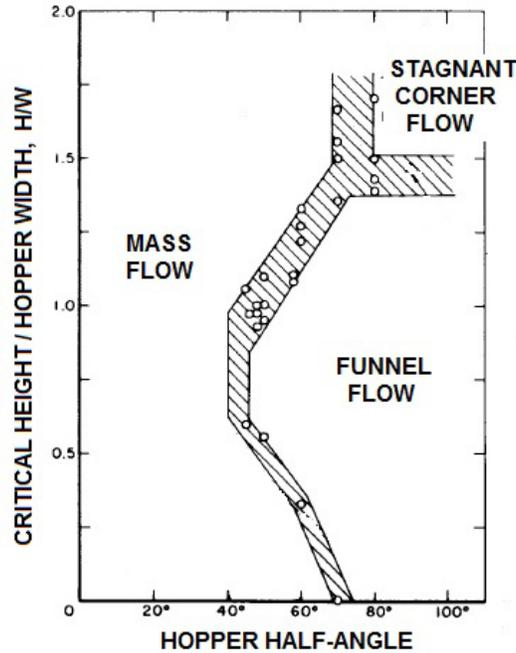
Figure 3: Flow regime map for sand in a planar hopper of width,  $W = 15.24\text{cm}$ , as a function of the material height in the hopper,  $H$ , and the hopper half-angle. From Nguyen *et al.* (1980).
