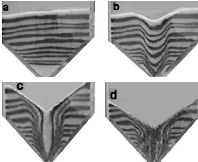
Figure 4: Photographs of funnel flow at four moments in time during discharge from a two-dimensional hopper. From Hunt *et al.* (1999).
