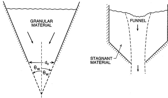
Figure 1: Some hopper geometries and notation. Left: a mass flow hopper. Right: funnel flow.
