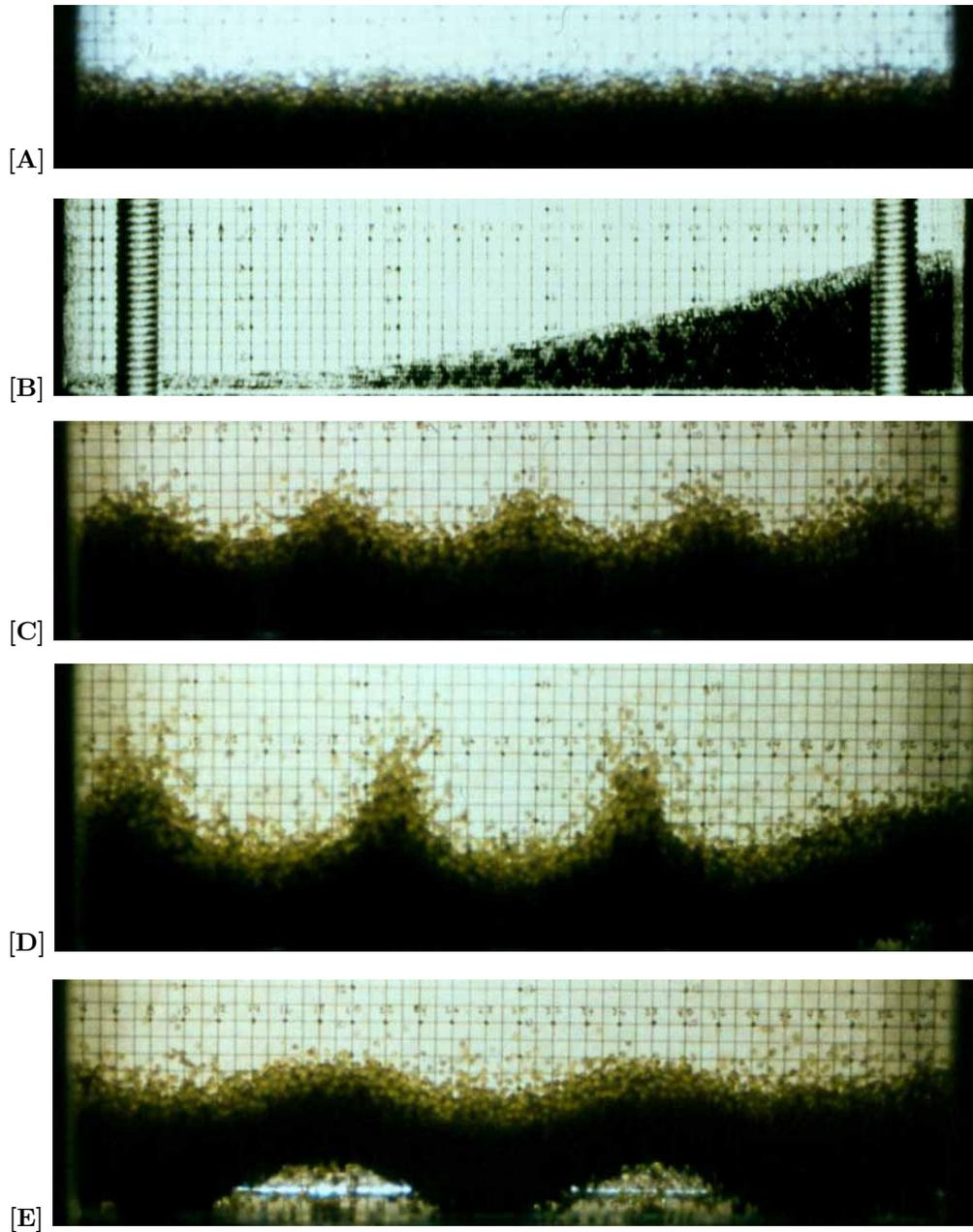
Figure 5: Flow patterns in a layer of 1.3mm diameter glass beads, 18 diameters deep, subject to vertical vibration: [A] At rest [B] Heaping [C]  $f/2$  waves at  $f = 20\text{Hz}$   $\Gamma = 3.3$  [D]  $f/4$  waves at  $f = 20\text{Hz}$   $\Gamma = 6.2$  [E] kinks at  $f = 30\text{Hz}$   $\Gamma = 8.5$ . Adapted from Wassgren (1997).
