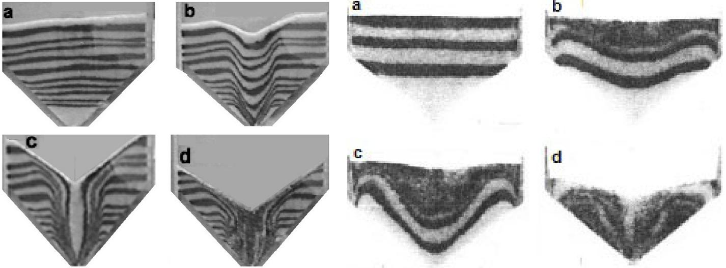
Figure 1: Four sequential images of the flow through a two-dimensional hopper: Left: Without imposed vibration. Right: With vertical vibration. Adapted from Hunt *et al.* (1999) and Wassgren *et al.* (2002).
