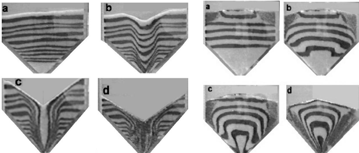
Figure 3: Four sequential images of the flow through a two-dimensional hopper subject to horizontal vibration: Left: Without imposed vibration. Right: With horizontal vibration. Adapted from Hunt *et al.* (1999).
