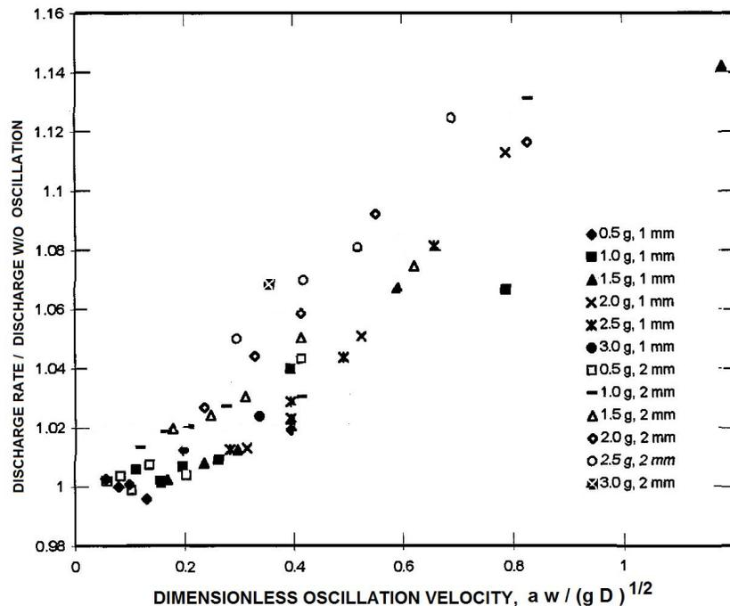
Figure 4: The dimensionless flow rate from a horizontally vibrating hopper as a function of the dimensionless oscillation velocity for two particle sizes (1mm and 2mm) and several oscillation accelerations as shown. Adapted from Hunt *et al.* (1999).
