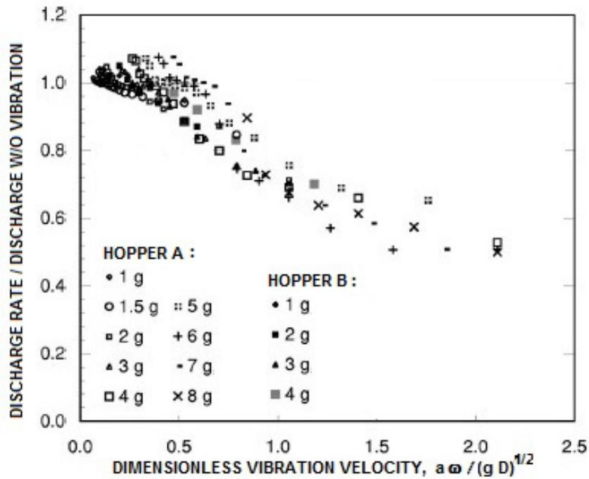
Figure 2: The dimensionless flow rate from a vertically vibrating hopper as a function of the dimensionless oscillation velocity for a number of vibration accelerations (in  $g$ ) and two different hoppers, A and B. Adapted from Wassgren *et al.* (2002).
