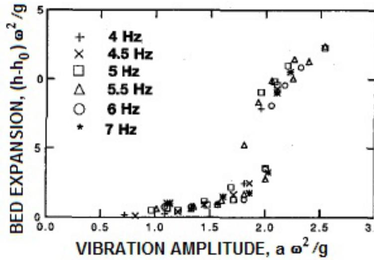
Figure 7: Example of the sudden expansion of a granular bed subject to vertically vibration. Adapted from Brennen *et al.* (1993).
