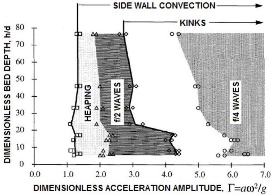
Figure 6: Flow regime chart for the vibration patterns due to vertical vibration of a deep bed of  $1.3\text{mm}$  diameter glass beads. Adapted from Wassgren (1997).
