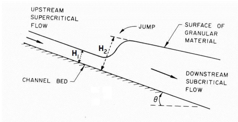
Figure 2: Notation for a granular flow hydraulic jump in an inclined chute. From Brennen *et al.* (1983).
