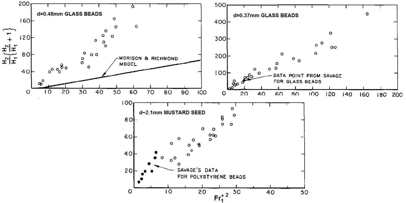
Figure 4: Experimental values of  $(H_2/H_1)[(H_2/H_1) + 1]$  plotted versus  $(Fr_1^*)^2$  for granular hydraulic jumps of three granular materials and a wide range of flow rates. Adapted from Brennen *et al.* (1983).
