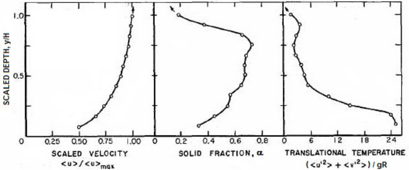
Figure 1: Typical profiles of velocity,  $u$ , solid fraction,  $\alpha$ , and granular temperature in a chute flow. From the simulations of Campbell and Brennen (1985b).
