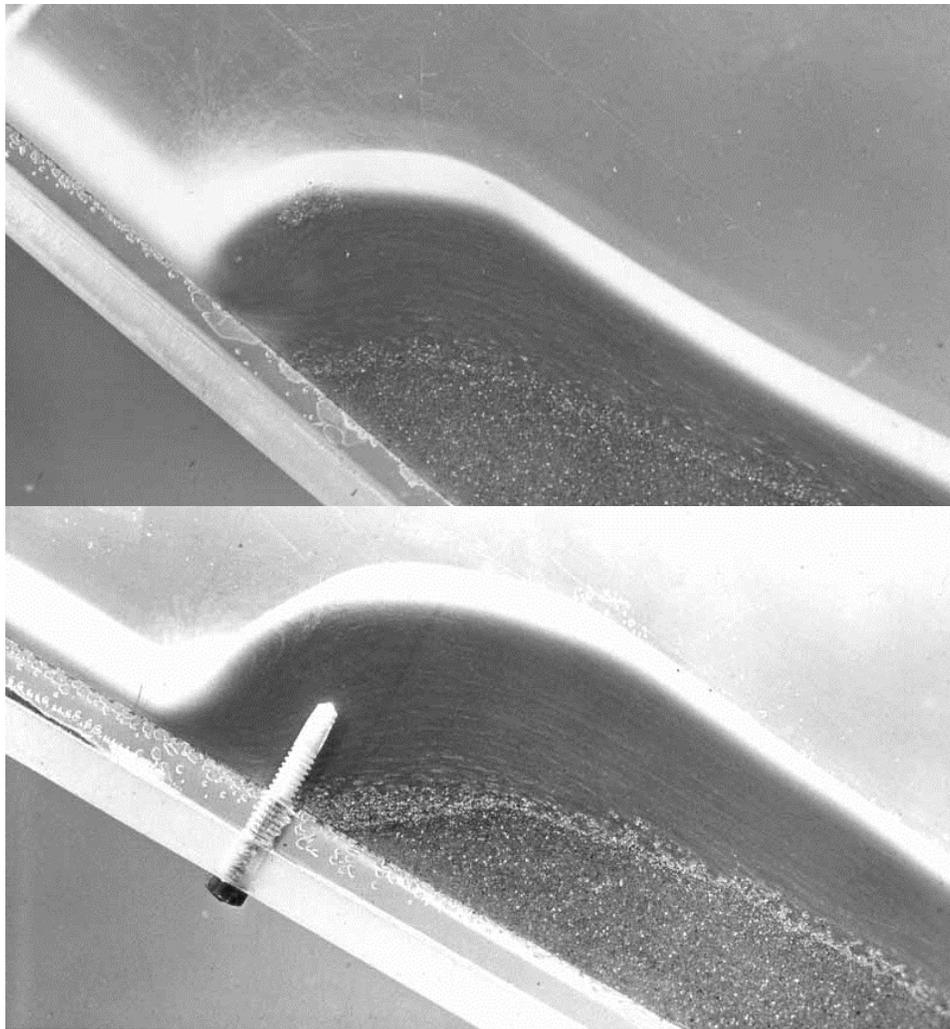
Figure 3: Examples of steady granular flow hydraulic jumps in an inclined chute. From Brennen *et al.* (1983).
