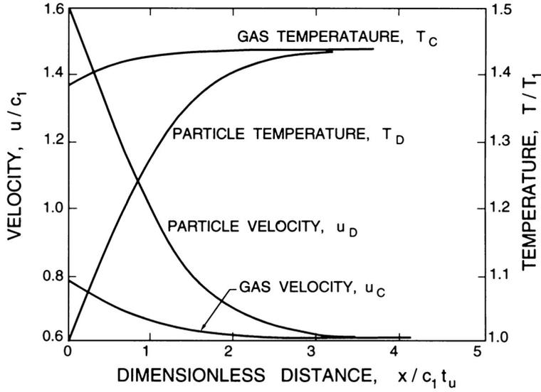
Figure 1: Typical structure of the relaxation zone in a shock wave in a dusty gas for  $M_1 = 1.6$ ,  $\gamma = 1.4$ ,  $\xi = 0.25$  and  $t_u/t_T = 1.0$ . In the non-dimensionalization,  $c_1$  is the upstream acoustic speed. Adapted from Marble (1970).
