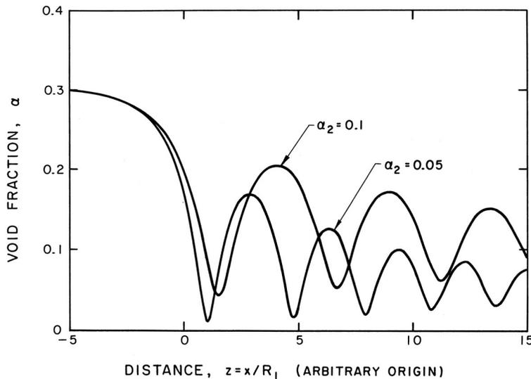
Figure 1: The typical structure of a shock wave in a bubbly mixture is illustrated by these examples for  $\alpha_1 = 0.3$ ,  $k = 1.4$ ,  $R_1(p_1 - p_V)/S \gg 1$ , and  $u_1 R_1/\nu_L = 100$ .
