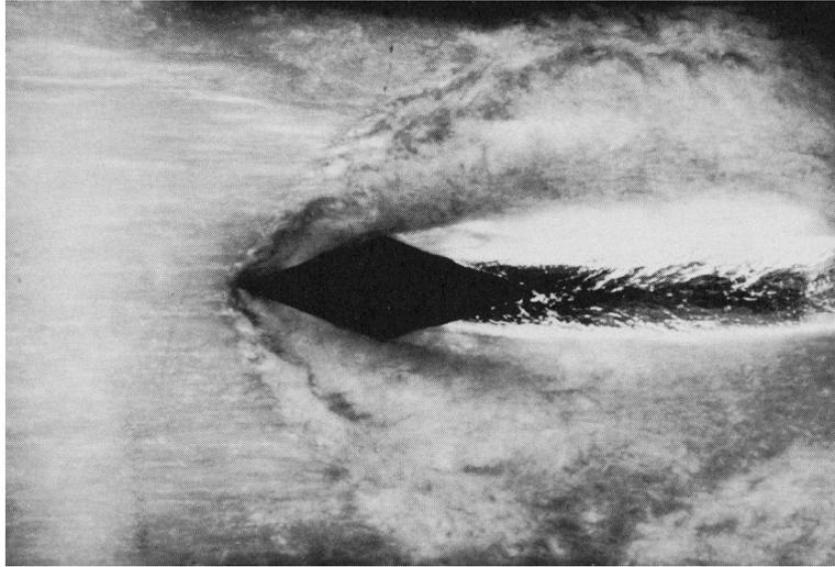
Figure 3: Supersonic bubbly flow past a  $20^\circ$  half-angle wedge at a Mach number of 4. Flow is from left to right. Photograph taken in supersonic bubbly flow tunnel (Eddington 1967) and reproduced with permission.
