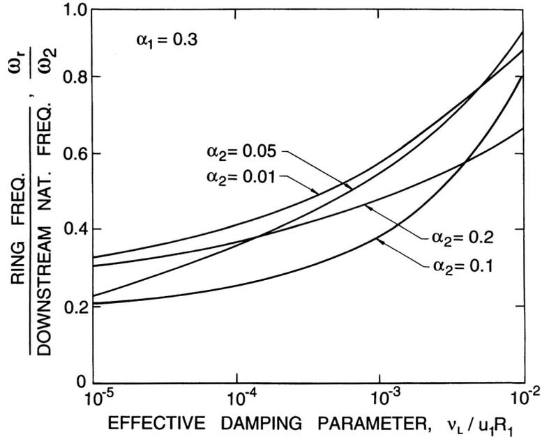
Figure 2: The ratio of the ring frequency downstream of a bubbly mixture shock to the natural frequency of the bubbles far downstream as a function of the effective damping parameter,  $\nu_L/u_1R_1$ , for  $\alpha_1 = 0.3$  and various downstream void fractions as indicated.
